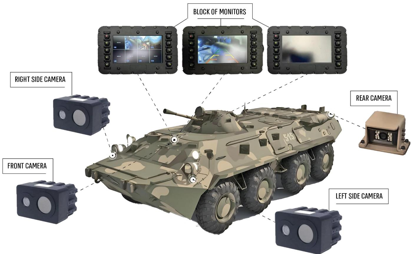
CHEETAH DVE Cameras System was designed to assist BTR driving when visibility is limited, in full darkness and all weather conditions, during day and night.
